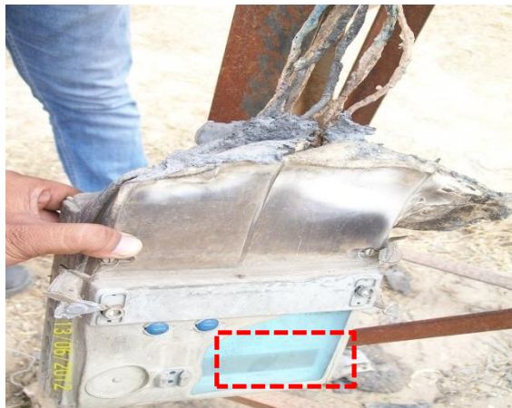
Defective meter installed in Kumher S/S in Bharatpur
