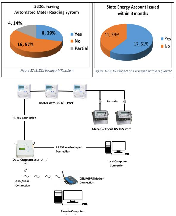
Figure 19: Schematic for Automatic Meter Reading System
