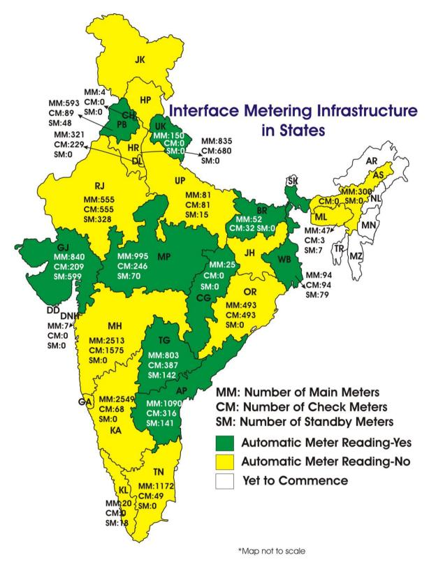
Figure 1: Metering Infrastructure at the Intra State level
