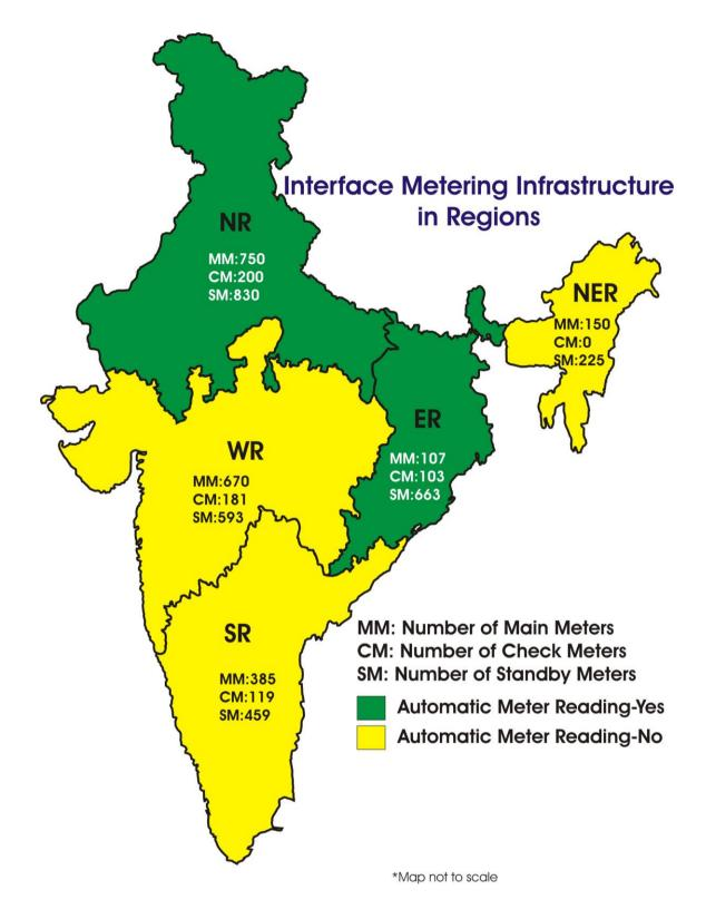
Figure 24: Metering Infrastructure at ISTS level
