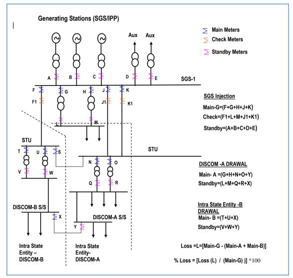
Figure 16: Recommended position of Energy Meters
