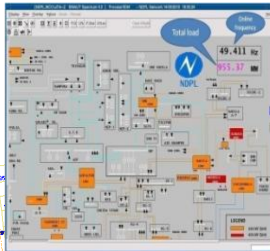
Monitoring of total load through SCADA
