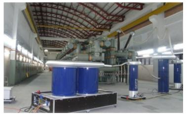
230kV Cables Oscillating Wave Test System
