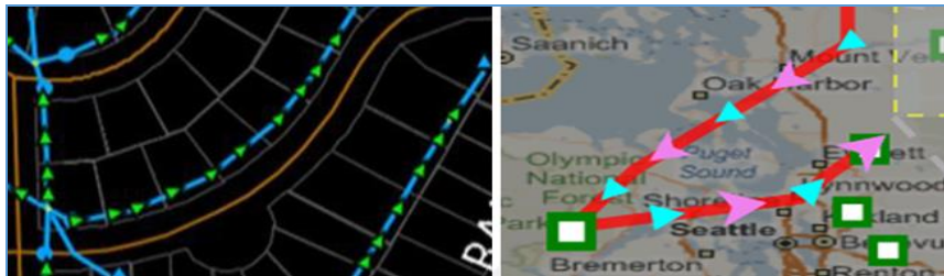
Figure 42: Example of Animated Power Flow Arrows in Transmission Lines
