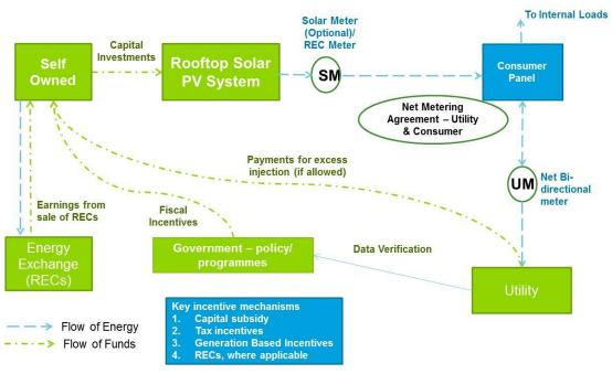
Figure 1: Self owned net-metering model
