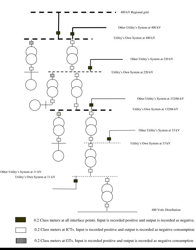
Loss at Particular Voltage level would be sum of energy recorded by all meters installed at that voltage
